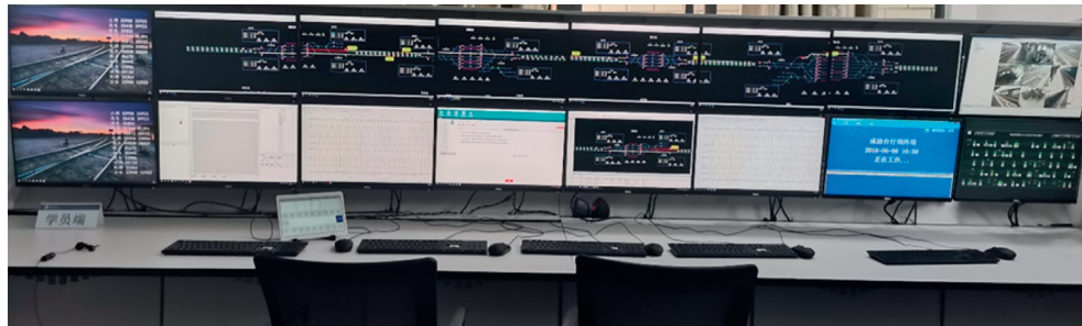
FIGURE 7: HSR dispatch simulator used to measure train delay time.
