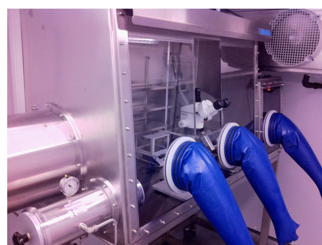
Figure 4. Glove box at -20°C equipped with the new polyurethane gloves.
