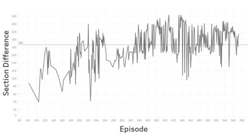
Fig. 22 Section difference at the end of a completed lap for Multi car SAC model on Altima VII during training
