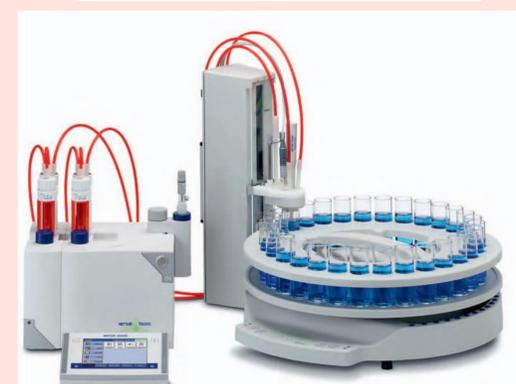
**Lower image:** Auto-titrator with Rondo sample changer (<http://2-lab.ru/files/catalog/7/632d0512bf55f53c253a04695f04a31c.pdf>)
