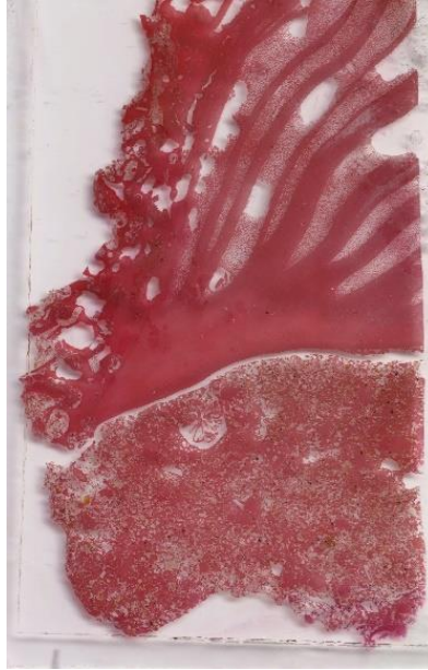
Figure 3. Thin section stained in Alizarin red
